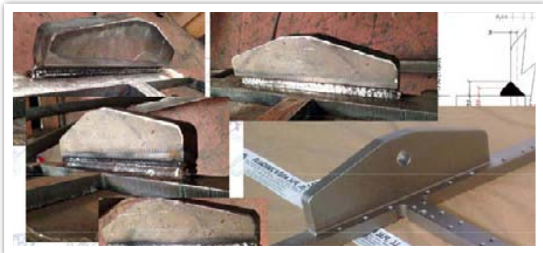
GMAW procedure: Semi-automatic manufactured parts for VLS MK-25 VLS Canister
