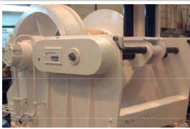
Tugboats winch, with automatic stevedore and emergency brake hydraulic system
