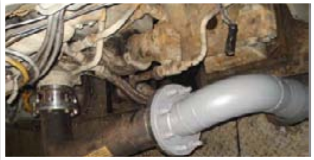
Tank Installation and hydraulic piping for fishing boat.
