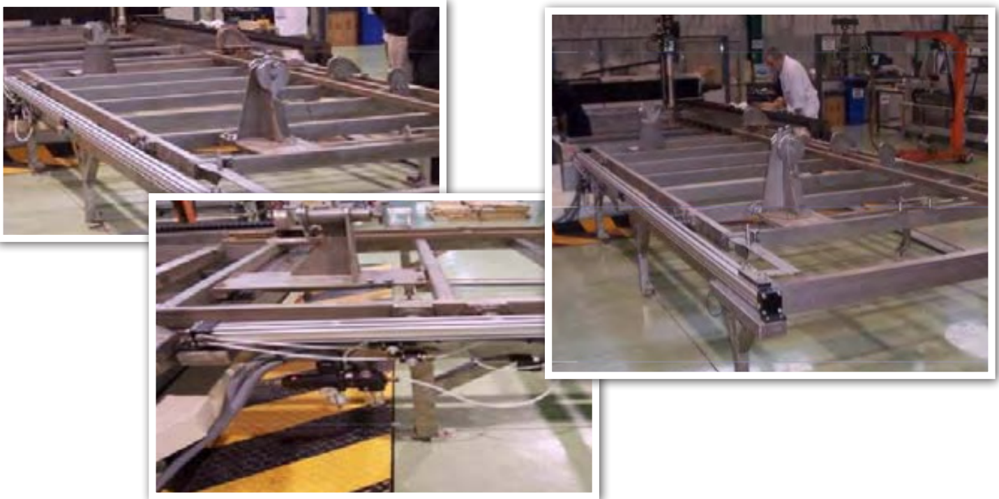
“Tecnautom” ultrasound table car for Military Airbus
