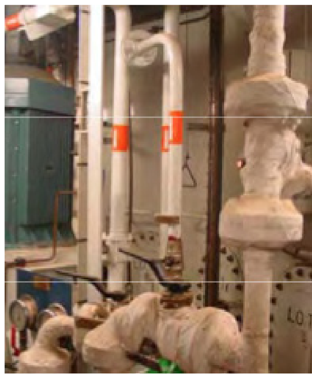
Deck Engine Hydraulic Piping. "Robert H. Boh" ship modification.
